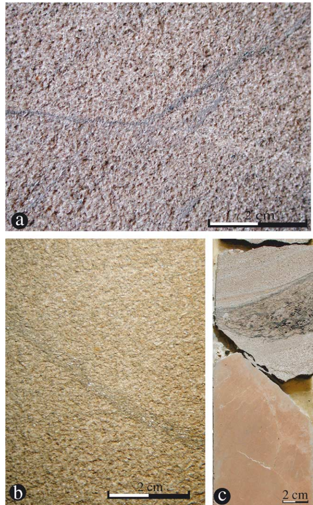
Fig. 11. (a) Deformation band from well L1. The band is a typical disaggregation band in the right part of the picture, changing to a phyllosilicate framework band in the left part of the picture. (b) Example of ~1 mm thick phyllosilicate framework band from the Huldra Field. Note the aligned platy minerals giving the bands a dark appearance. Well L1. (c) Minor fault in well L3. Note drag in the hanging wall. Orientation analysis indicates that this fault has a southerly strike and dips about 40° to the west.
